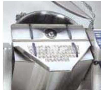
Two-part strainer plate (300 l). Additional part is used when necessary.
